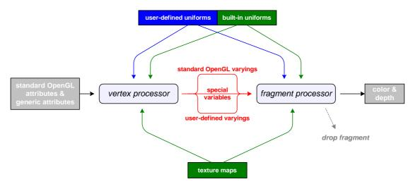
Figure 2. Input, intermediate data flow and output of vertex and fragment shaders
