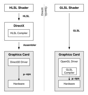
Figure 4. Shader compilation of HLSL and GLSL
